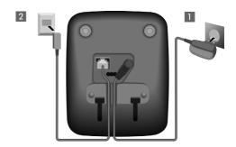
◆ Only use the mains adapter and phone cord **supplied**. Pin connections on telephone cables can vary (pin connections → page 44).
